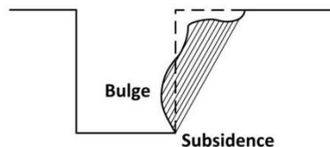
An unsupported excavation can also create an unbalanced stress in the soil, which, in turn, causes subsidence (sinking) at the surface and bulging of the vertical face of the trench. If left unsupported, this condition can cause the face of the excavation to collapse and trap workers in the excavation.
