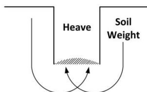
Bottom heaving or squeezing is caused by the downward pressure created by the weight of adjoining soil. This pressure causes a bulge in the bottom of the cut, as illustrated in the drawing above. Heaving and squeezing can occur even when shoring or shielding has been properly installed.
