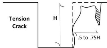
Tension cracks usually form on the top of the ground parallel to the sides of an excavation. They typically form at a horizontal distance of  $1/2$  (.5) to  $3/4$  (.75) times the depth of the trench, measured from the vertical face of the trench.
