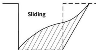
Tension cracks can eventually lead to sliding of the soil into the excavation, as illustrated in this drawing. Tension cracks can also lead to sloughing or unravelling (crumbling or running) of the soil down the face of the excavation.
