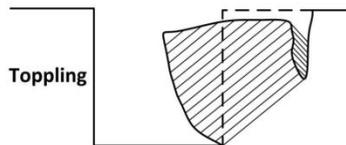
Tension cracks can also lead to toppling of the soil. Toppling occurs when the trench's vertical face breaks off along the tension crack line and topples into the excavation. Any of these conditions can result in the worker being trapped inside the excavation.
