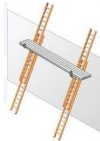
Ladder Jack Scaffold
