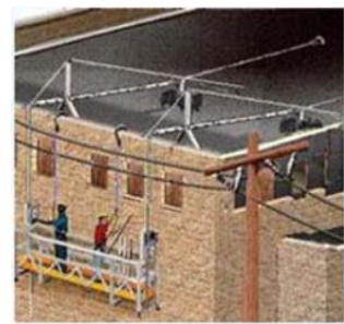
Two-point Swing Stage Scaffold
