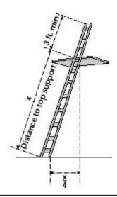
Proper 3-foot side-rail extension at top of ladder, and best angle for portable extension ladder set against a wall or other supporting structure.
