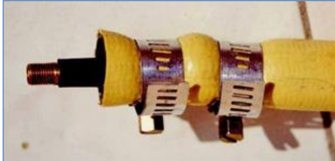
Water Hose Clamps Used on Compressed Air Hose NOT Approved for Use
